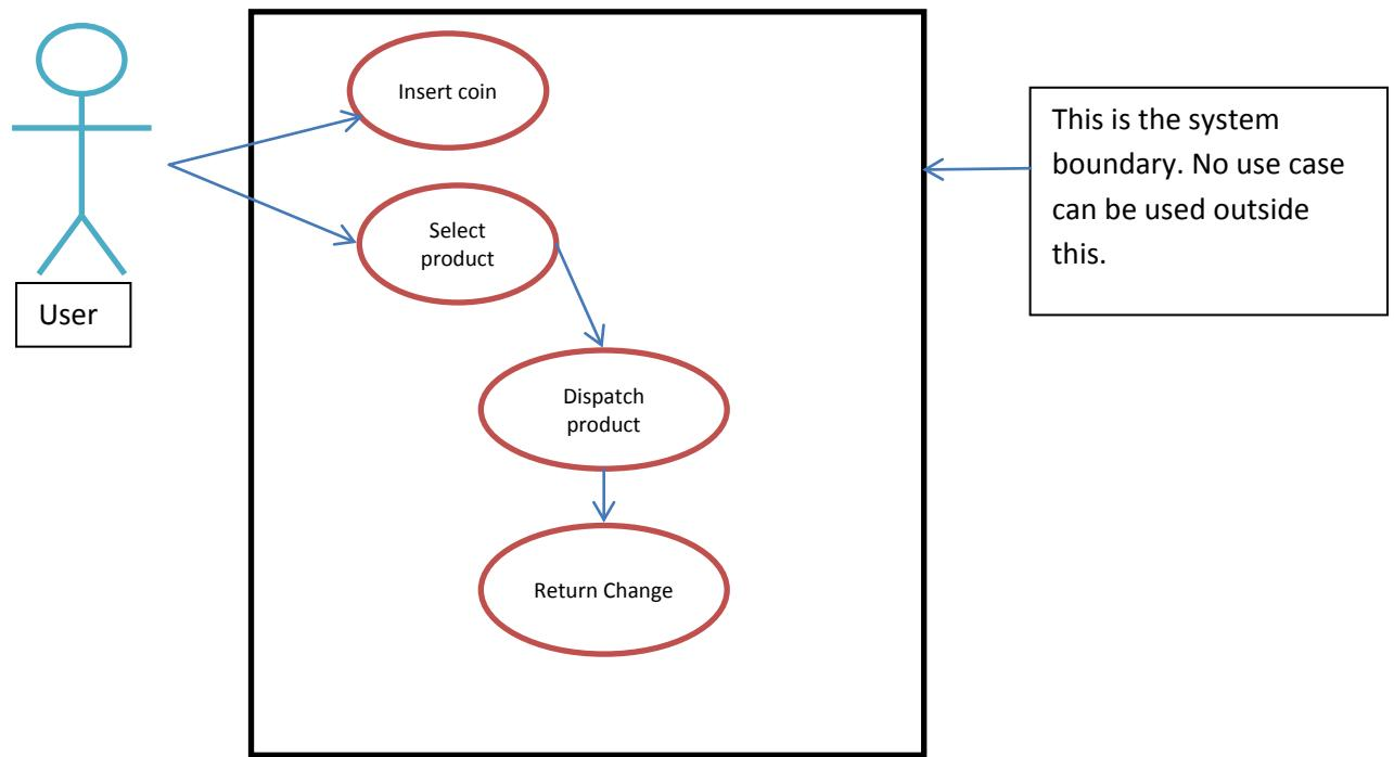
Here we have a simple USE CASE DIAGRAM of a vending machine. The user here has an option to insert coin and then to choose a product. Once the machine verified the amount and the choice from the user it can dispatch the product and return any change left to the user. Since the system outputs the return to the user we won't need to show an arrow back to the user.
